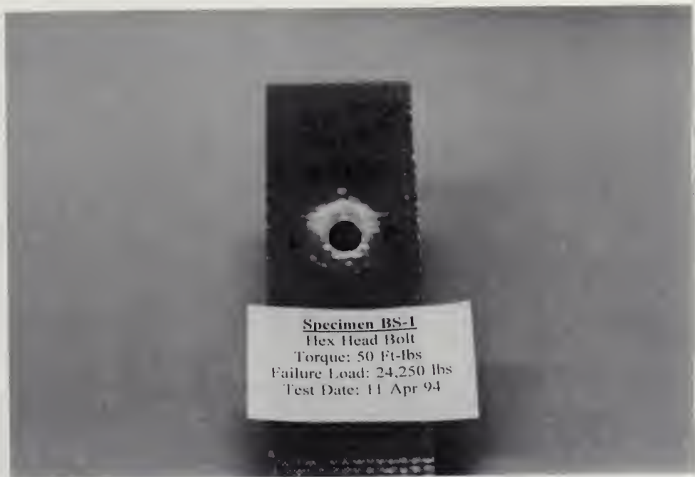
Specimen BS-1, Hex Head Bolt, 50 ft-lbs torque. View of outer GRP surface showing delamination, moderate brooming and hole deformation.
